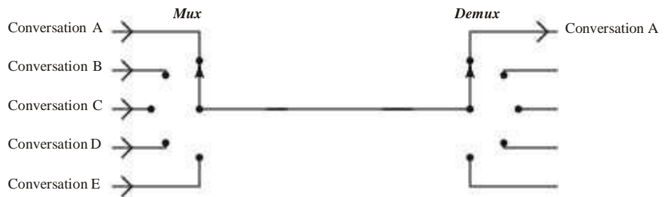
Fig. 4.29 Multiplexer and Demultiplexer
