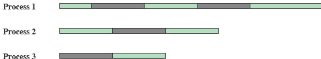
(b) Interleaving and overlapping (multiprocessing; two processors)
